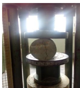
Fig 6: split tensile strength test
