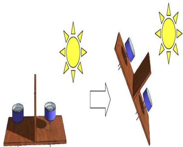
**Figure 1. Sensor response once a shadow is cast on one LDR**
