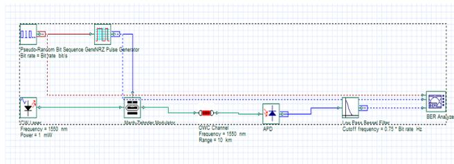
The length of the wireless optical channel is differed. To produce the optical signs we have utilized a CW laser source, Mach-Zehnder modulators, RZ signal generator and a sinusoidal electrical sign generator.
