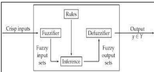
Fig-1: A block diagram of fuzzy Logic System Fuzzifier
