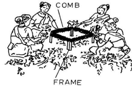
Figure 5. Comb Type Stripper
