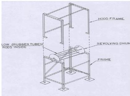
Figure 4. Drum Type Pod Stripper
