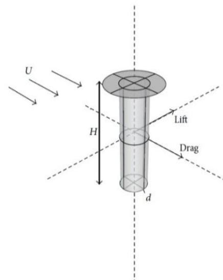
Fig.1 Forces acting on Flettner Rotor
