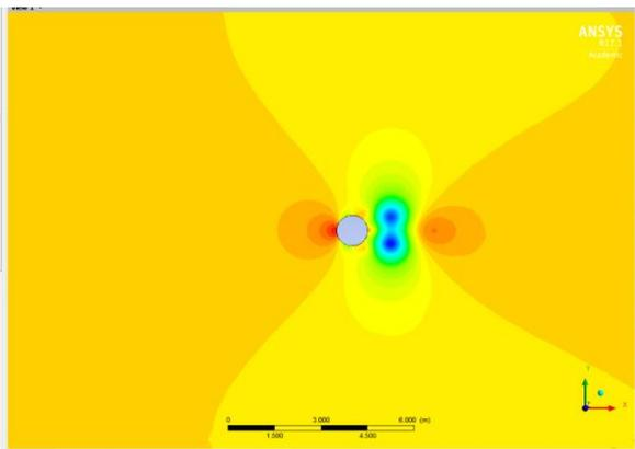
Fig.7 represents Stationary cylinder with fluid inlet speed 7m/s
