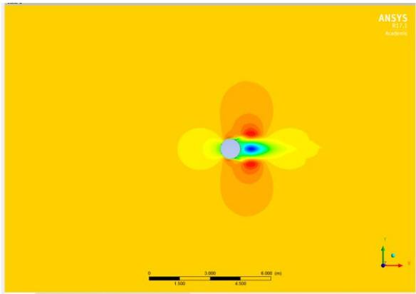
Fig.6 represents Stationary cylinder with fluid inlet speed 7m/s
