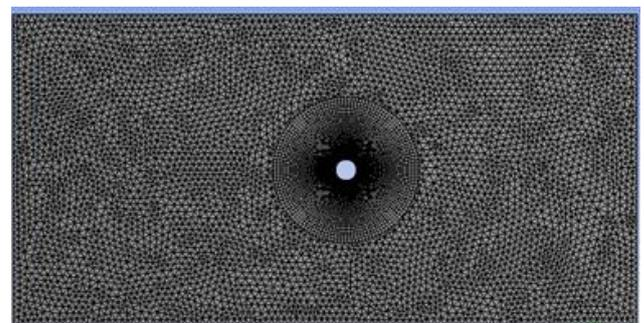
Fig .5 shows Meshing around 2-D Cylinder
