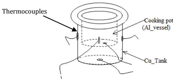
Fig -2: Details of cooking pan and position of thermocouples
