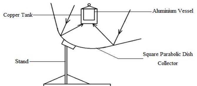
**Fig -1:** Experimental setup of solar cooker
