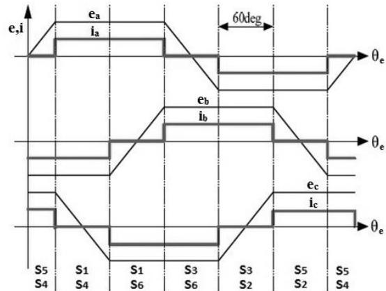
Fig. 3: Back emf and phase current waveforms
