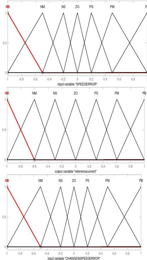
Fig. 2: Fuzzy membership functions for (a) speed error (b) change in speed error (c) reference current
