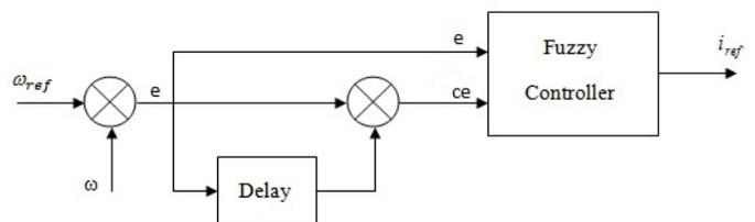
Fig. 1. Block diagram of fuzzy control system
