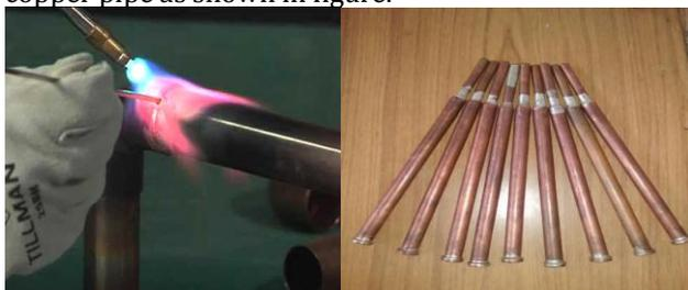
**Fig -1:** a) Brazing process b) Before pinching
