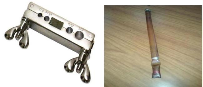
**Fig -2:** Pinching equipment b) after pinched copper tube
