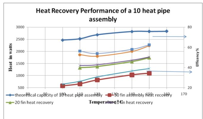
Chart -1: Heat Recovery Performance of a 10 heat pipe assembly
