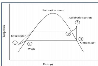
Fig -4: Thermodynamic cycle
