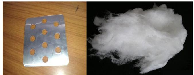
**Fig -3:** a) Aluminum fin sheet b) Ceramic wool
