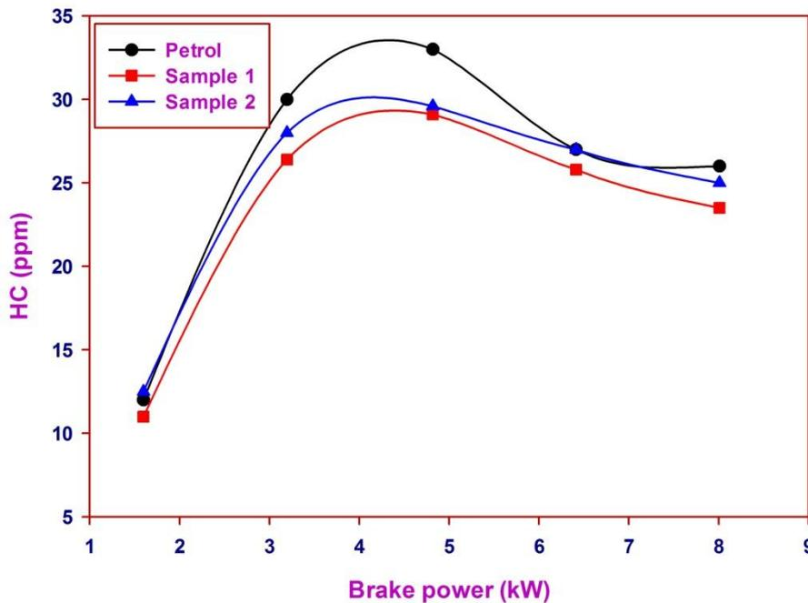
**Figure 6** Variations of HC emission with brake power
