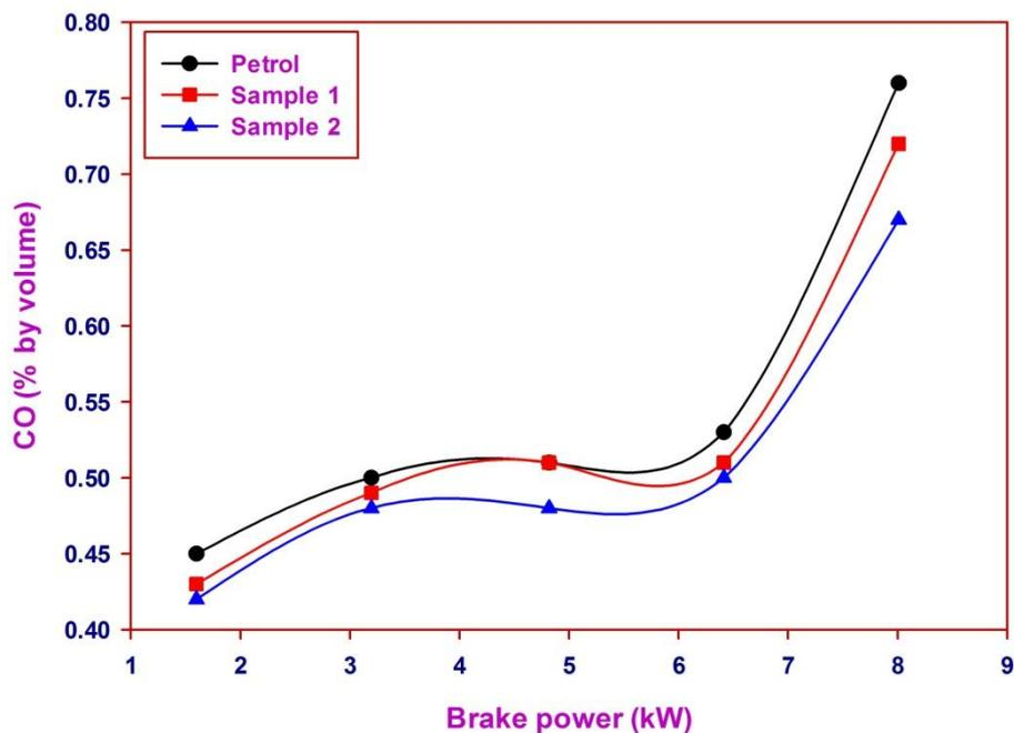
Figure 5 Variations of CO with brake power
