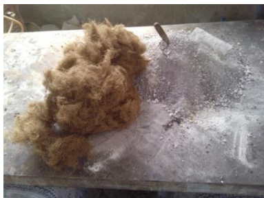
Fig.3 Dry mixing of BCS, Lime & Coir
