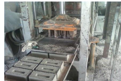
Fig.4 Casting of brick in Hydraulic Compression Machine
