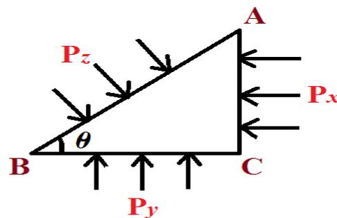
**Fig -2:** Element of Liquid
