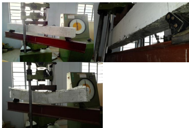
Fig -4: Testing Of Beam With Fibre (Soffit), (Soffit+ U) Wrapping
