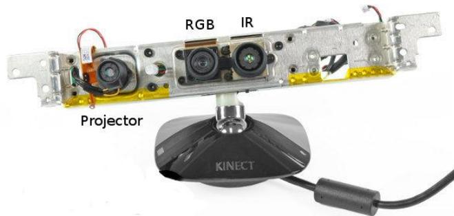
Kinect consists of Infra-red (IR) projector, IR camera and RGB camera
