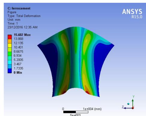
**Fig.6 Total Deformation of Ferrocement**
