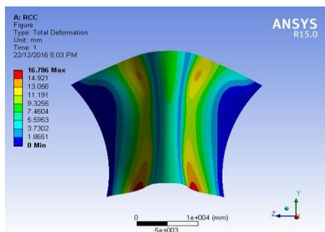
**Fig.3 Total Deformation of RCC**
