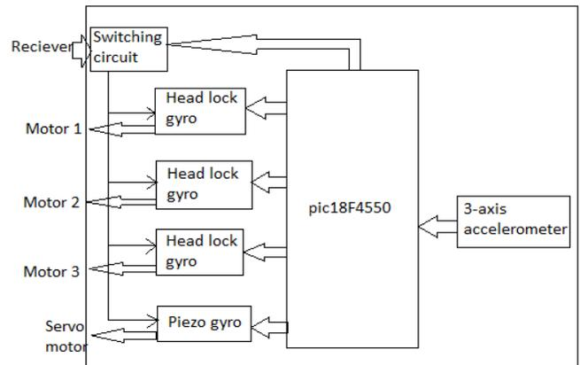
Fig 2: Architecture of flight control board
