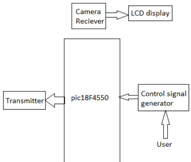
Fig 3: Ground station block diagram
