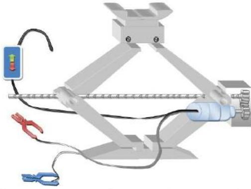
Figure 4: Assembly Diagram of a powered jack
