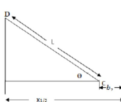
Figure 2: Free body diagram of link CD
