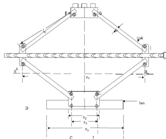
Figure 1: Schematic diagram of the powered jack
