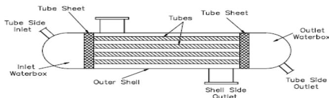
**Fig-1:** shell and tube heat exchanger [5]
