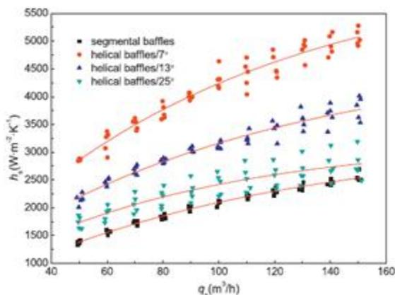
Chart-1: Heat transfer coefficient with volume rate for different baffle helix angle. [8]
