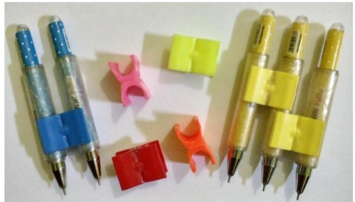
**Fig 5: Multi Instrument Writing Device for Concurrent Signatures**
