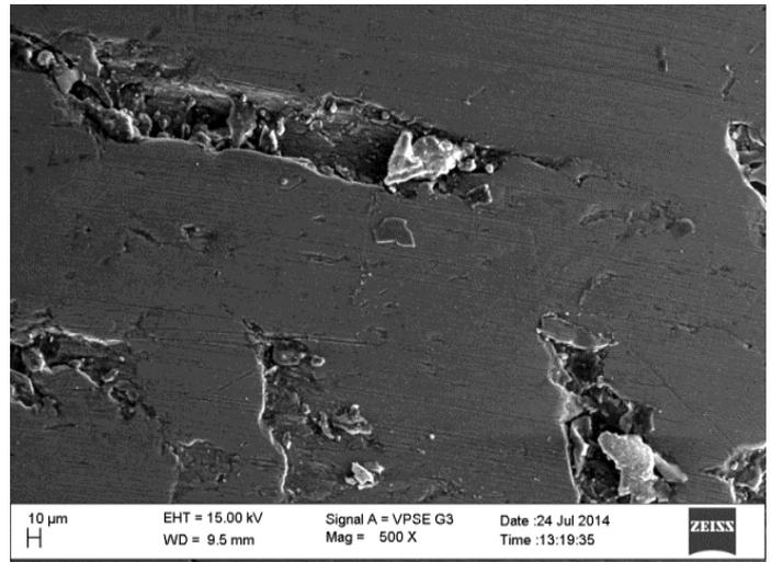
Fig. 6. SEM Microstructure of Al6061 with 5%SiC and 5% Graphite [48]
