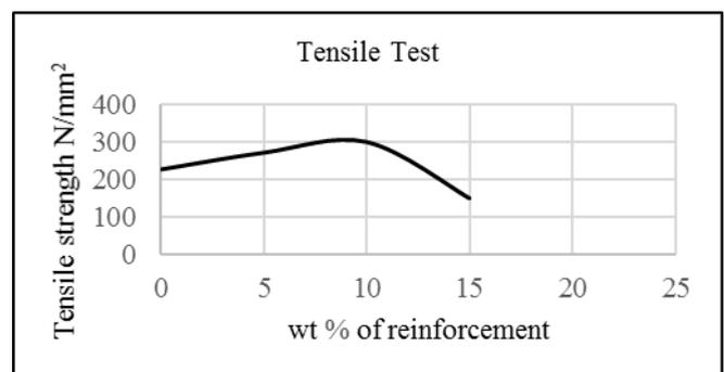
**Chart 2. Tensile strength variation with wt.% of fly ash [17]**
