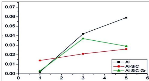
Chart 6. Variation of Load (x-axis) vs Wear rate (y-axis) for Al359 [3]
