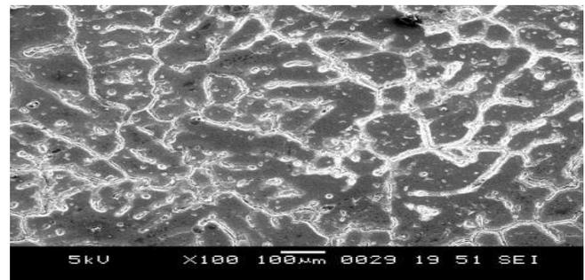
**Fig. 3. Microstructure of Al6061 with 20% weight fraction of fly ash [11]**
