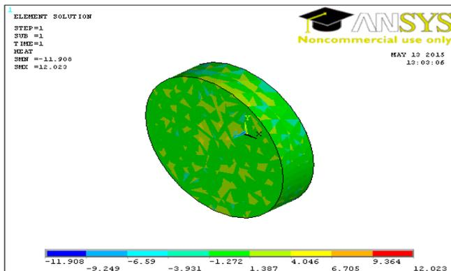
Fig. 5. Heat flow Al6061 with 5% SiC and 5% Graphite [48]
