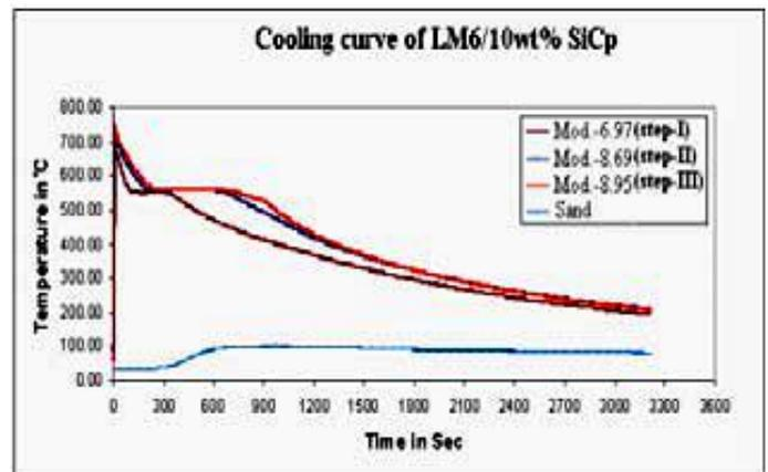
Chart 9. Cooling Curve graph of LM6 with 10wt% SiC at different modulus of casting [50]
