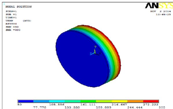
Fig. 4. Temperature distribution of Al6061 with 5% SiC and 5% Graphite [48]
