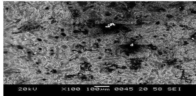
**Fig 2. Microstructure of Al 6061 with 15% weight fraction of fly ash [8]**
