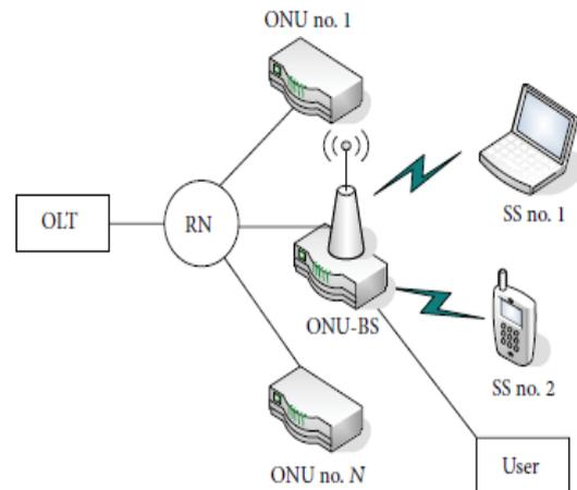
Figure 2: R&F Wi-Fi access network architecture: PON and its wireless extension ONU-BS
