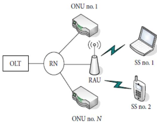
Figure 1: RoF Wi-Fi access network architecture: PON and its wireless extension RAU
