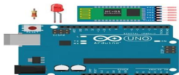
Diagram 2.4.1: arduino with Bluetooth device[1]
