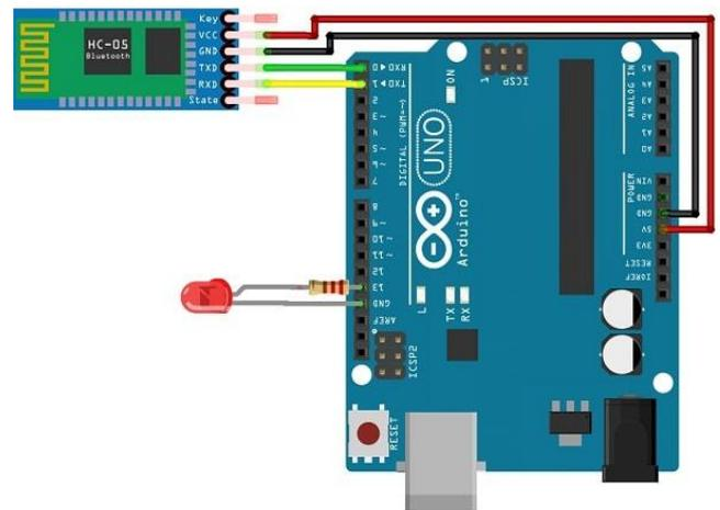
Diagram 3.1 :Arduino with Bluetooth connectivity[1]
