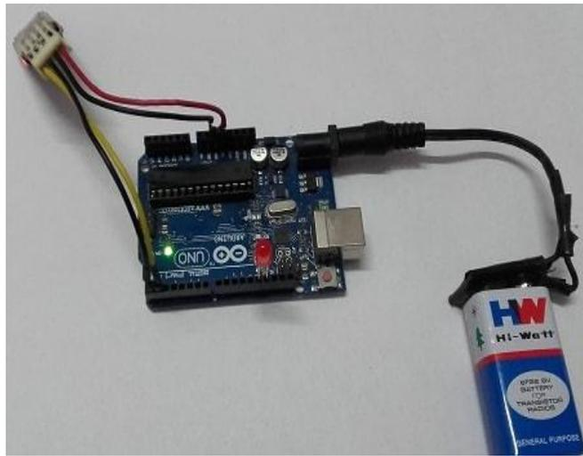
Diagram 3.2. : connect the Bluetooth module to the Arduino using jumper wires and a connector[1].
