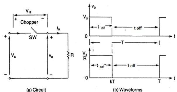
Fig-1: DC Chopper Circuit And Waveforms
