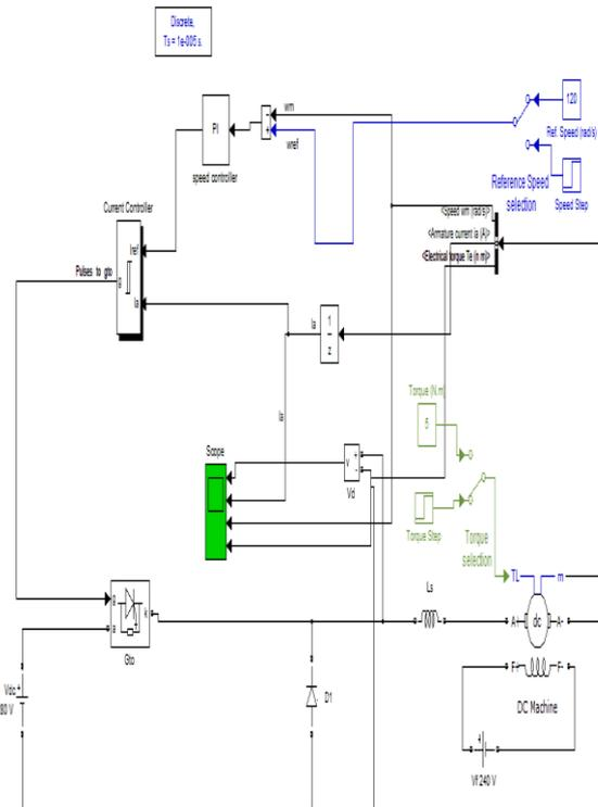
Fig. 4: MATLAB Simulation Model
