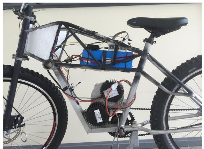
Fig-4: The ride monitoring module mounted to an E-Bike
