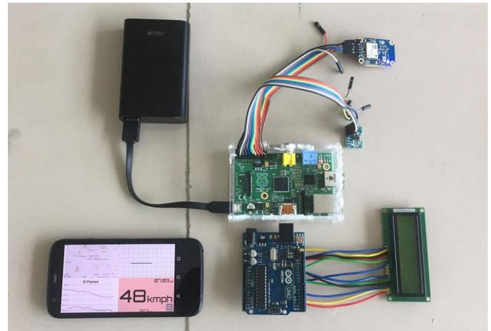
Fig-3: Raspberry pi connections with sensors
