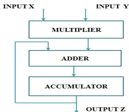
Fig-1: Block diagram of MAC unit
