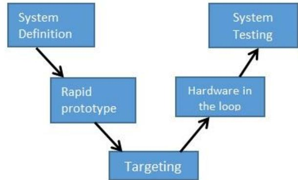
Fig.02: Embedded System Design Cycle (“V” Diagram)
