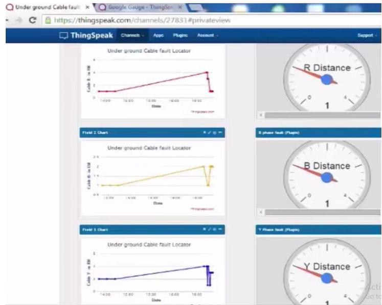
**Fig.06:** Graphical Representation of 1 Km Fault in R, B, Y cables.
