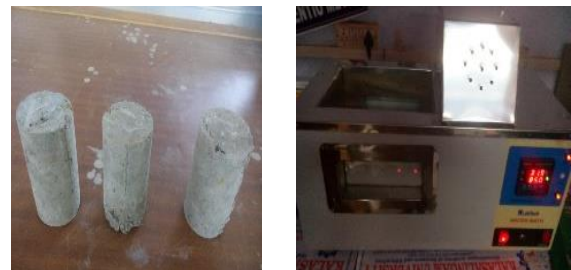
FIG 5 Cylinder of size 100mm diameter x 50mm height, Water bath.
