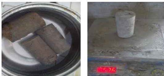
FIG 6 Concrete specimens on water bath and specimens while weighing
