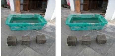
FIG 3 Concrete cube of size 70mm x 70mm and 1% Sulphuric acid diluted in distilled water.
