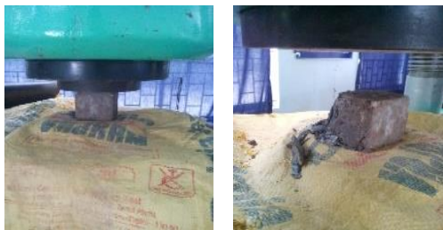
FIG 4 Concrete cubes before and after testing in compression machine
