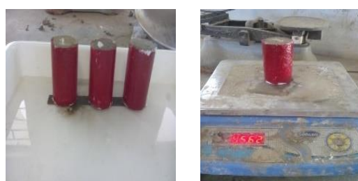
FIG 8 Sorptivity test setup and weighing of specimens
