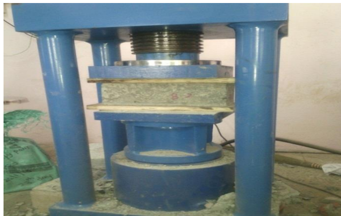
Figure-3: Compression test on papercrete bricks
