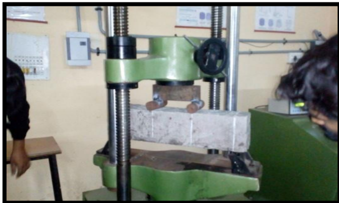
Fig.7 Flexural strength testing by UTM
