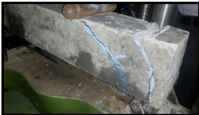
Fig.8 Pattern of cracks due to testing
