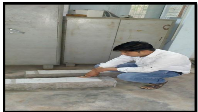
Fig. 4 beam specimen after 28 days curing
