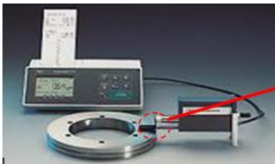
Fig -2: Roughness Measurement Instrument (Perthometer)
