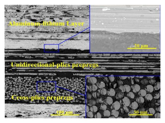
Figure 1: The interface between the aluminum-lithium layer and prepares [17]
