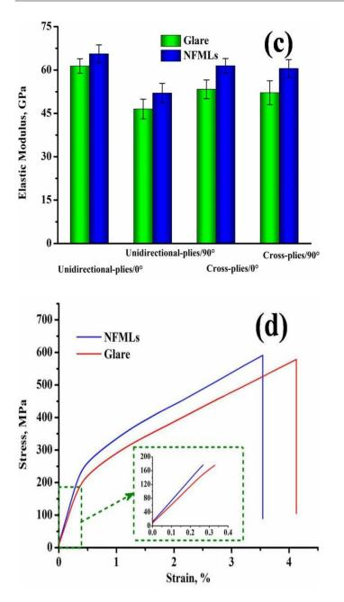
Figure 2: Tensile and flexural properties of NFMLs and Glare: (a) tensile strength; (b) flexural strength, (c) elastic modulus; (d) the tensile stress-strain curves (crossplies/0<sup>0</sup>) [17]
