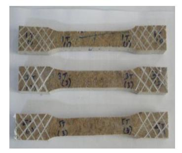
Figure 3: Aluminum-GFRP Composite specimen
