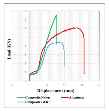
Figure 4: Load Displacement diagram for various composite material
