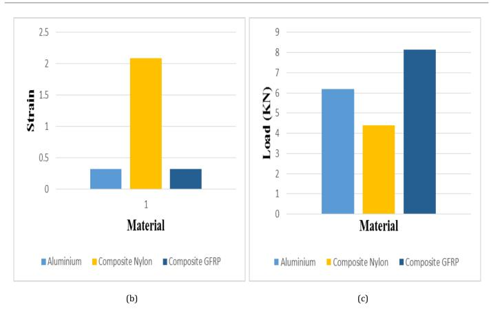
Figure 5: Comparision of Composite material (a) Tensile strength, (b) Strain, (c) bearing load
