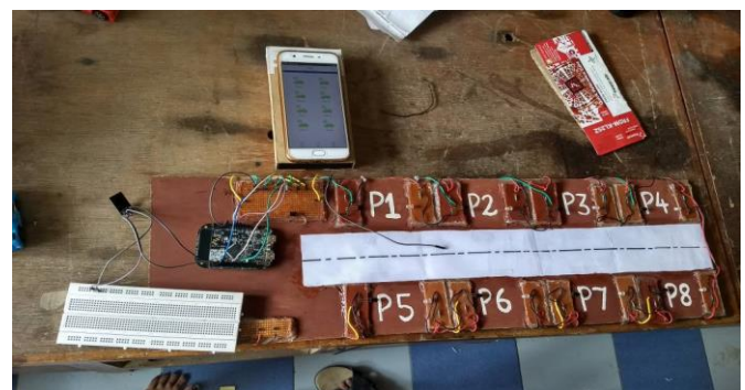
Fig -5: Hardware implementation of prototype (When all parking slots are vacant)
