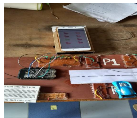
Fig -6: Hardware implementation of prototype (When car is parked on slot no. 5 i.e. P5)
