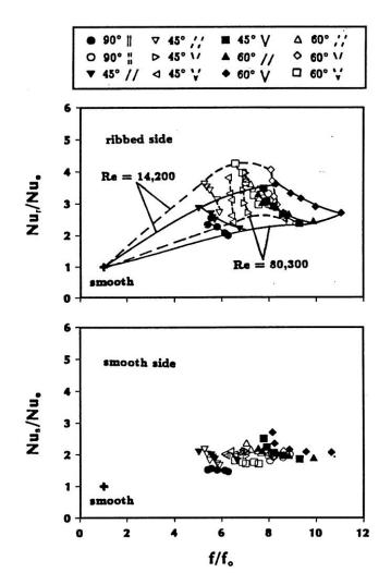
Figure-2 : Comparison of heat-transfer between broken and continuous ribs [6].
