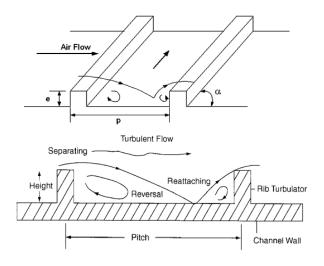
Figure-1 : Flow in a channel with rib turbulators
