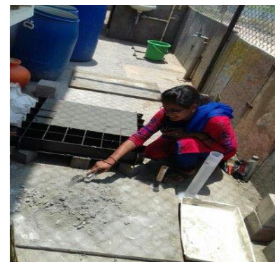
Fig1: Portion mixing of Nano-Silica with super plasticizer, water and fine aggregate.
