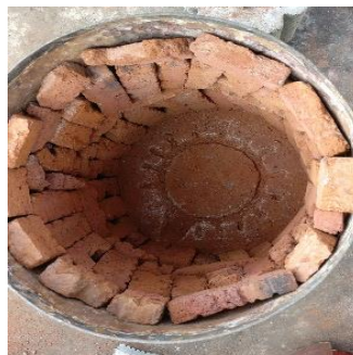
Fig no: 1. Brick insulated Furnace
