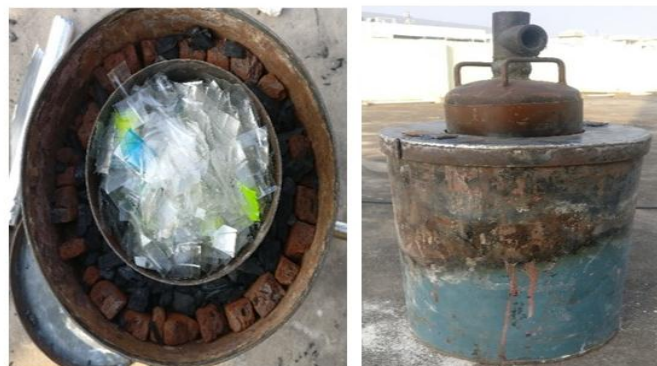
Fig no: 2. Reactor unit
