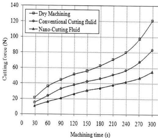
Fig 4.—Variation of cutting force with machining time for dry machining and machining with conventional and nano-cutting fluids
