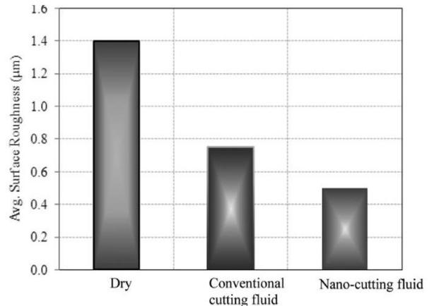
Fig 5.—Variation of average surface roughness while dry machining and machining with conventional and nano-cutting fluid.
