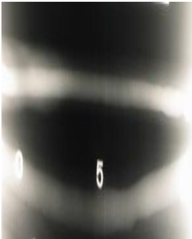
Fig.4. Double wall double image radiograph (Defect free) of a pipe butt weld. Note the IQI, identification numbers and position markers.
