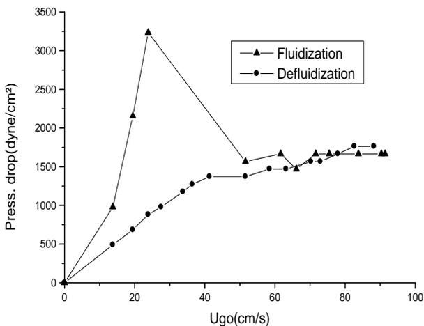
**Plot -2:** Effect of superficial gas velocity on pressure drop in conical bed for flour
