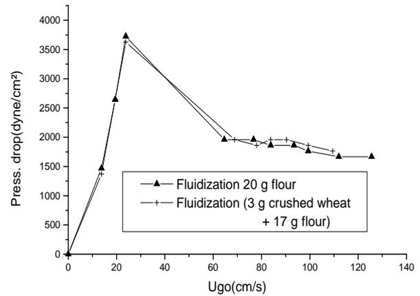
**Plot -7:** Variation of bed pressure drop with superficial velocity showing effect of additive
