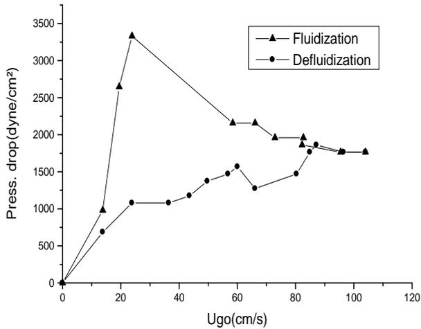
**Plot -1:** Effect of superficial gas velocity on pressure drop in conical bed for flour
