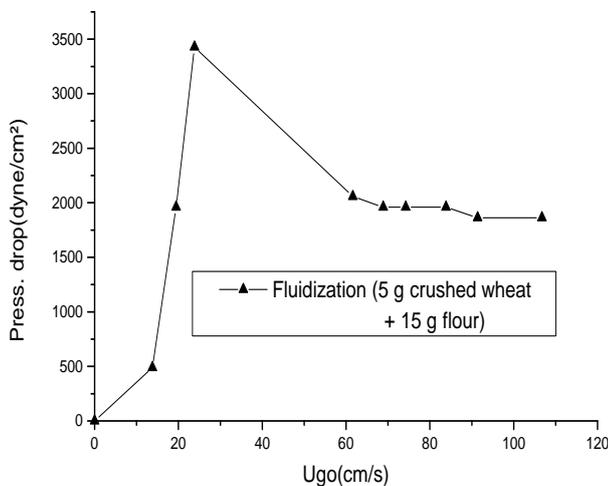
**Plot -6:** Variation of bed pressure drop with superficial velocity showing effect of additive
