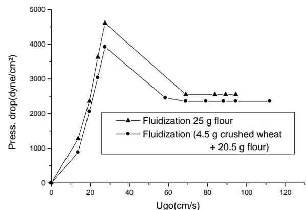
**Plot -8:** Variation of bed pressure drop with superficial velocity showing effect of additive
