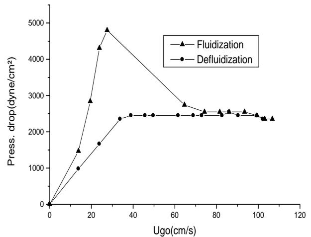
**Plot -4:** Effect of superficial gas velocity on pressure drop in conical bed for flour (bed height of 6 cm)
