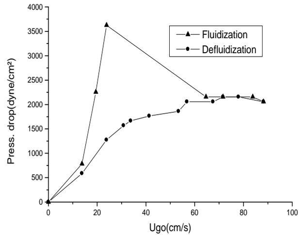
**Plot -3:** Effect of superficial gas velocity on pressure drop in conical bed for flour
