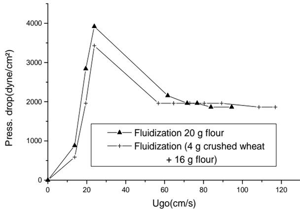
**Plot -5:** Variation of bed pressure drop with superficial velocity showing effect of additive
