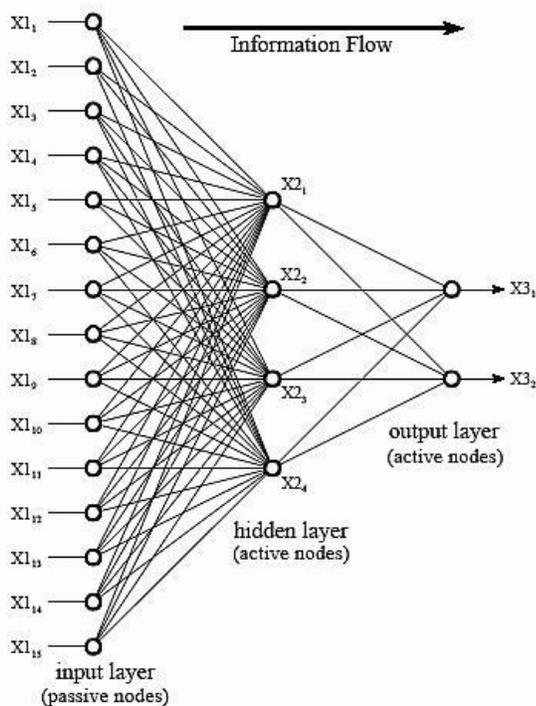
Their multiple outputs. In correlation, the nodes of both hidden and output layer are functioning. This means that they modify the given data as depicted. The variables X1-15 hold the data to be processed.
