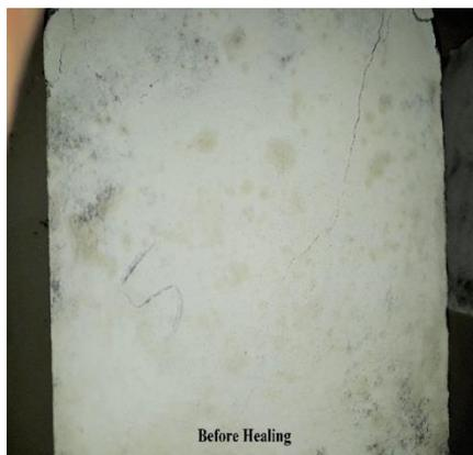
**Fig.1- Cracked Specimen**
