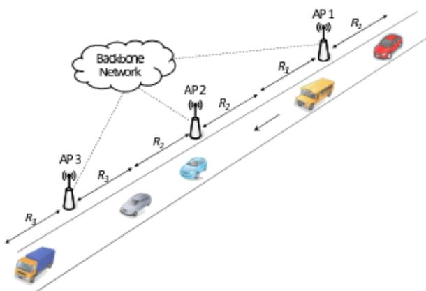
Fig. 1. Drive-thru vehicle-to-roadside (V2R) communications with multiple APs
