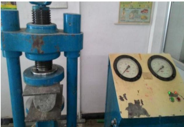
**Fig.3. Flexural Strength test in UTM**
