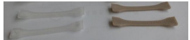
Fig.16 3D printed sample of dumbbell shape of neat PP and PP-K10 on adhesive strips coated heated bed.
