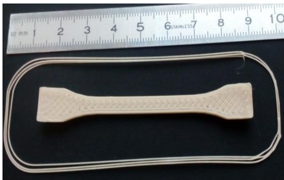
Fig.7 3D printed sample of K10-HP dumbbell and microfilaments.
