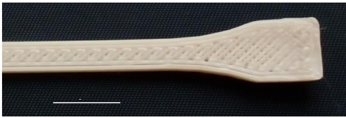
Fig.14 3D printed dumbbell sample of K10-HP (x3).
