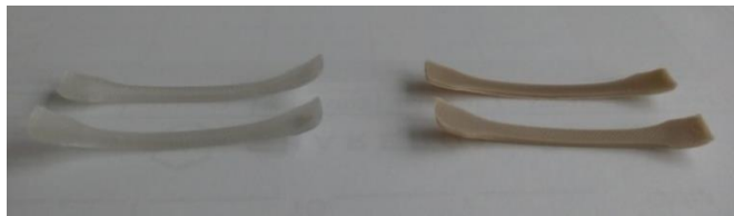
Fig.15 3D printed sample of dumbbell shape of neat HP and K10-HP on a heated bed.
