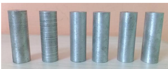
Fig -3.1: Cold upsetting test specimen before compression
