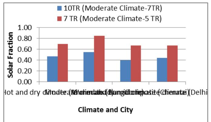
Fig 4 Comparison of Solar Fraction (PVArea-90 m<sup>2</sup>)
