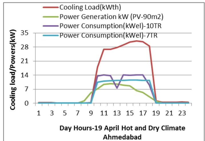
Fig: 5 Day Night profile of Cooling Load, Power Generation, and Consumption
