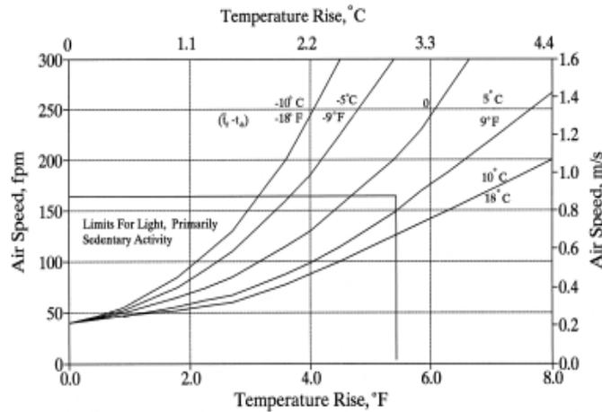
Fig 2 Air speed required offset increased temperature [ASHRAE 55-2004]
