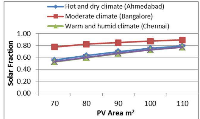
Fig. 3 Variation of Solar Fraction with PV area
