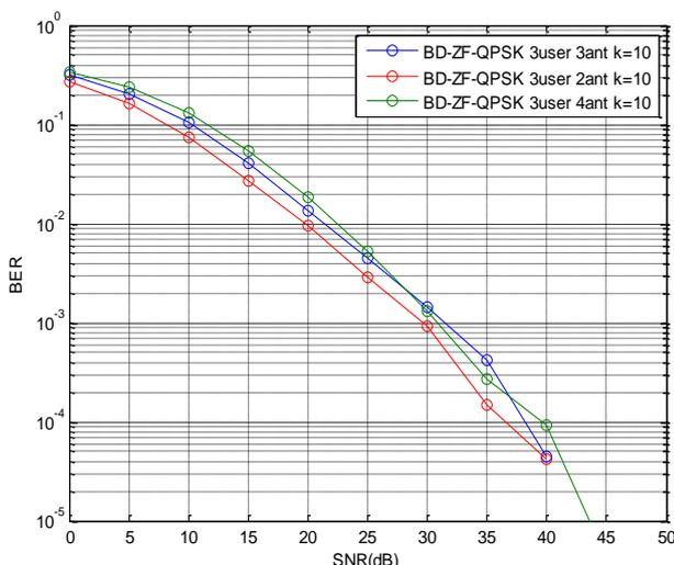
**Fig -3:** BER performance of MU-MIMO system using BD at the transmitter and ZF detection at 3 receivers each equipped with 2,3 and 4 receive antennas.
