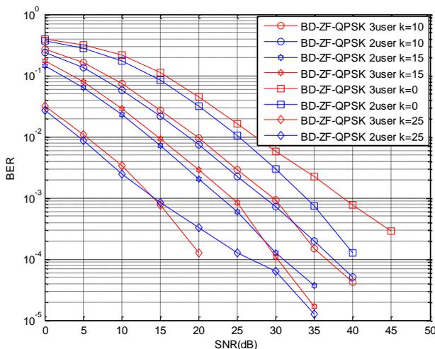
**Fig -2:** BER performance of MU-MIMO system using BD at the transmitter and ZF detection at 3 receivers each equipped with 2,3 and 4 receive antennas.
