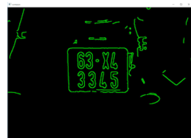
Fig. 4 Extraction of ROI using green bounding box
