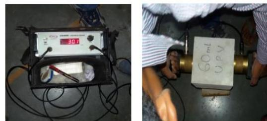
Fig: Test of bacterial concrete samples using Ultrasonic Pulse Velocity Machine.
