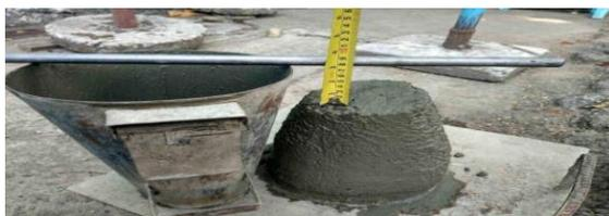
Fig: Slump Cone Test
