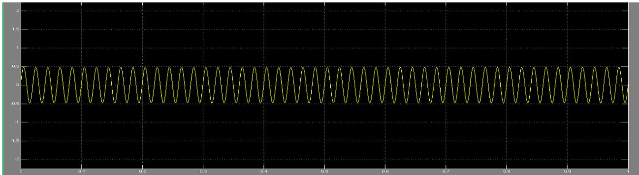
**Fig.(4d):** Load voltage of phase-A during single-phase fault
