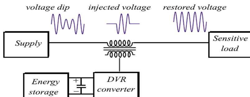
Fig2. Operating Principle of DVR
