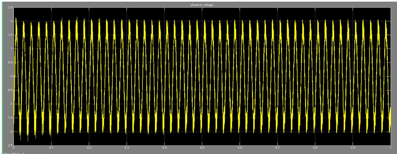
**Fig.(4 e):** Load voltage of phase-A after the DVR operation on single-phase fault
