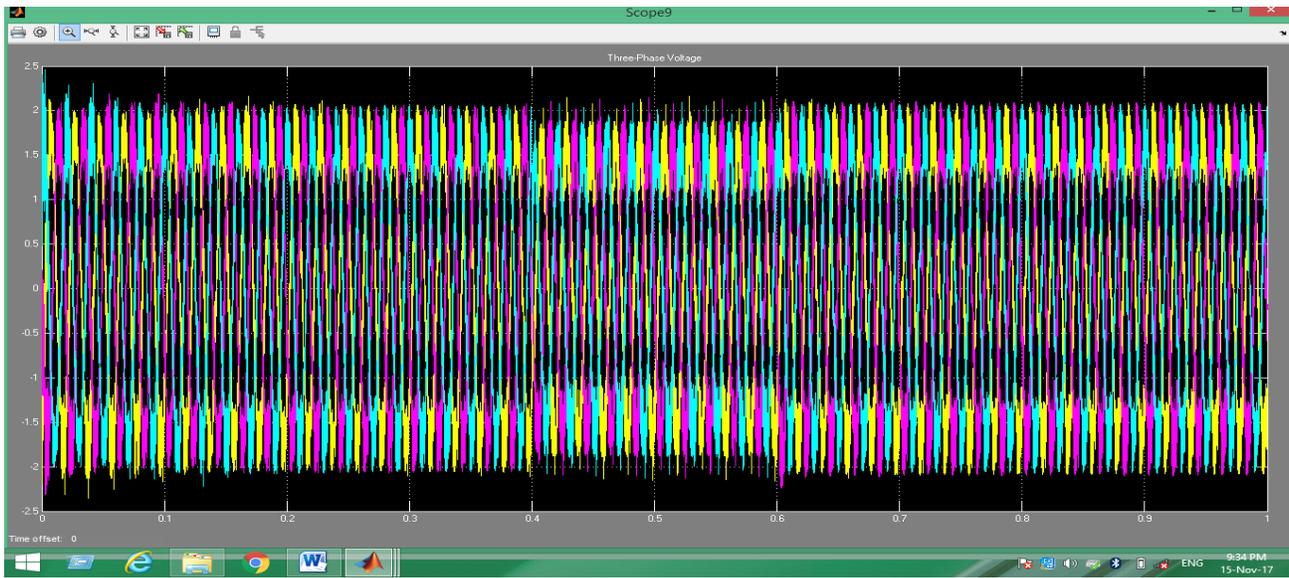
**Fig.(4c):** Load voltage after the DVR operation on three-phase fault
