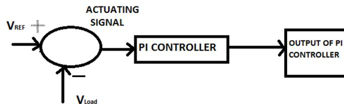
Fig3. Operation of PI controller
