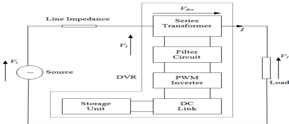
Fig. (1) A Simplified Block Diagram of Dynamic Voltage Restorer (DVR)
