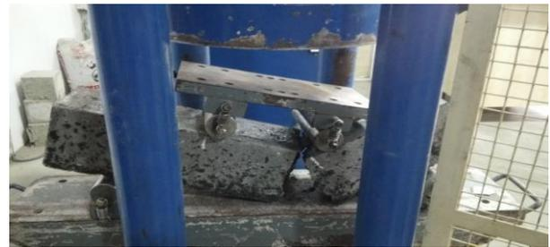
Fig.-1 Flexural beam test of specimen
